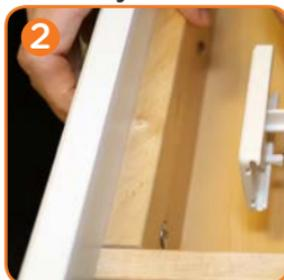
3 Remove the adhesive protective liner on the Mounting Plate. Slowly push the drawer in until the Mounting Plate sticks to the drawer box. Now reach in with your fingers and press firmly on the Mounting Plate against the drawer box for at least 30 seconds.
