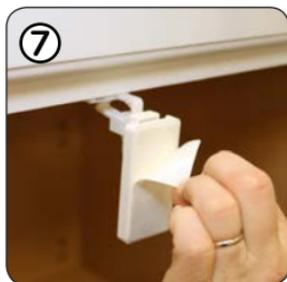
8. Carefully close the door until Mounting Plate sticks to it. Open door and press Mounting Plate firmly against the door for 30 seconds. Do not use a screw as it may penetrate the front of the door. Remove Perfect-Installation Tool.
